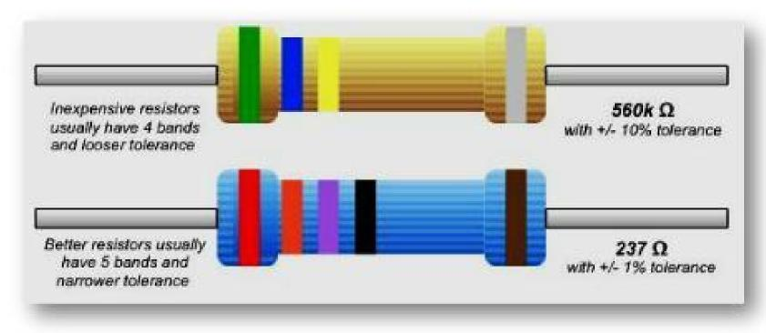
If your resistor has four color bands, turn the resistor so that the gold or silver band is on the right hand side or the end with more bands should point left.
