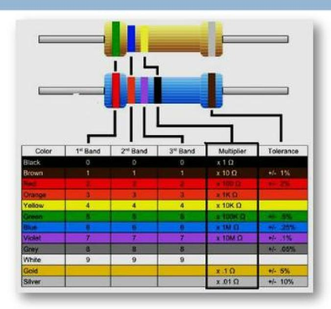
The third band denotes the 3<sup>rd</sup> digit – for a 5 band Resistor. In this case - 5 band its '7'. So the value of the 5 band resistor is 237 Ohms as its multiplier digit is '0'.
