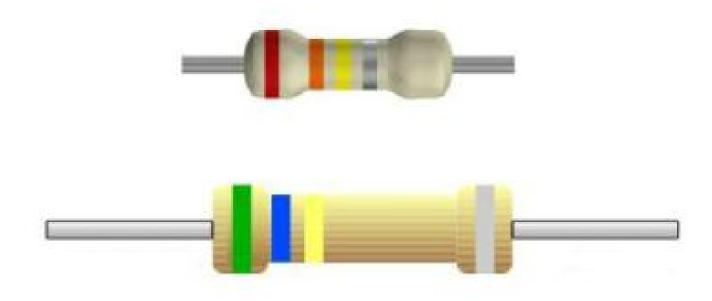
The first band is now on the left hand side. This represents the first digit. Based on the color make a note of the digit. In this case - 4 band its '5' and for 5 band its '2'.
