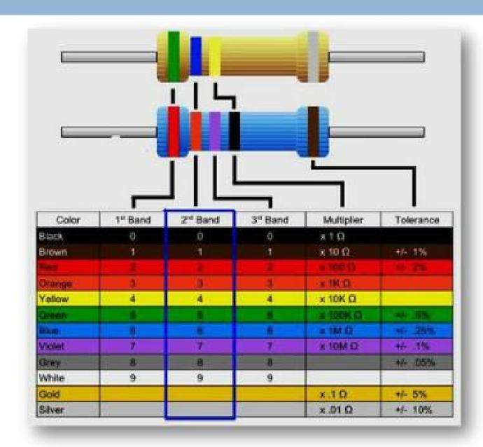
The third band divulges how many zeros to add/divide to the first two numbers – for a 4 band Resistor. In this case - 4 band its '4' zeroes to be added. So value is 560K.
